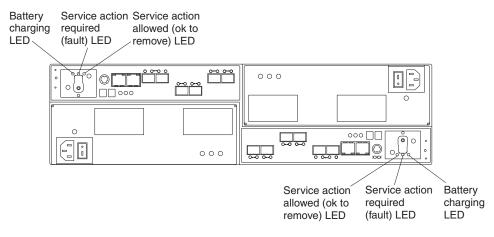
Figure 68. Battery unit LEDs
